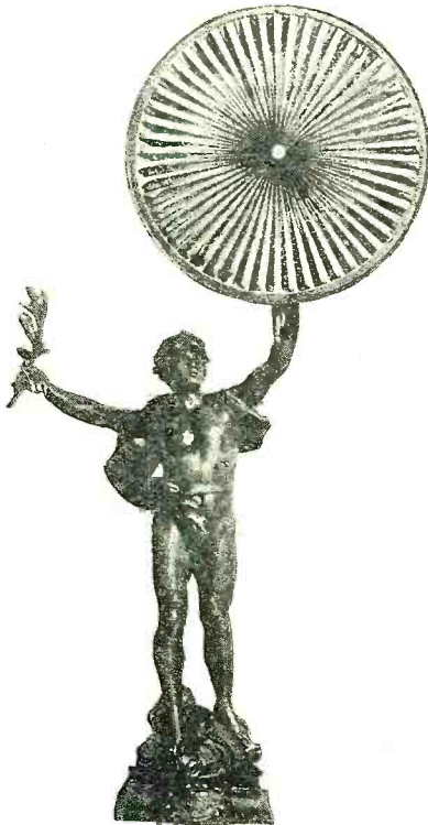
That the aesthetic side of radio is not being neglected is shown by this artistic loud speaker recently placed upon the English market. The diaphragm of the speaker is made of pleated parchment, the phone unit being supported close behind it.
